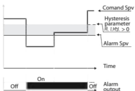
Absolute alarm referred to the command setpoint. Hysteresis value greater than "0" (Par. 20 R.I.HY > 0). The command setpoint can be modified using the serial port RS485 commands (word 1001).
