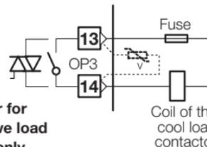
Coil of the cool load contactor
