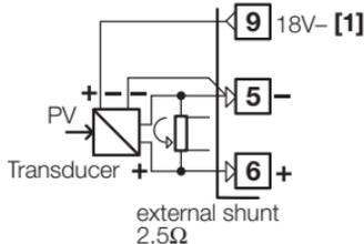
[1] Auxiliary power supply for external transmitter 18Vdc  $\pm 20\%$  /30mA max. without short circuit protection
