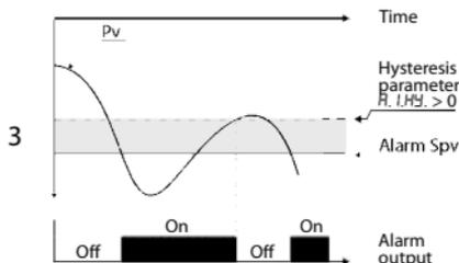
Absolute alarm with controller in cooling functioning (Par.7  $R_{CT.E}$  selected  $COOL$ ) and hysteresis value greater than "0" (Par.29  $R.I.HY. > 0$ ).\*
