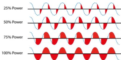
Using a no zero-crossing SSR, the ATR227 synchronizes with the power supply voltage (necessarily AC) and determines when to activate the output to create the right chocking.
