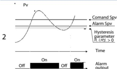
Upper deviation alarm value of alarm setpoint less than "0" and hysteresis value greater than "0" (Par.29  $R.I.H.Y. > 0$ ).\*\*
