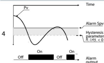
Absolute alarm with controller in cooling functioning (Par.7  $R_{CT.E}$  selected  $COOL$ ) and hysteresis value less than "0" (Par.29  $R.I.HY. < 0$ ).\*
