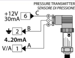
For linear signals 0/4..20 mA with three-wires sensors.
