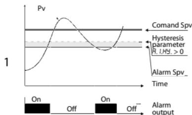
Lower deviation alarm value of alarm setpoint greater than "0" and hysteresis value greater than "0" (Par.29 R.L.H.Y. > 0).\*\*
