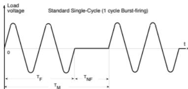
For a percentage less than 66%, SSR output firing takes place as in the "Burst fire" mode (see *bS.t.F.*)
