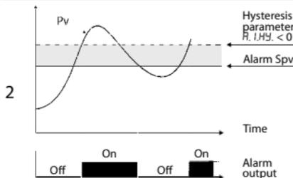
Absolute alarm with controller in heating functioning (Par.7  $R_{CT.E}$  selected  $HEAT$ ) and hysteresis value less than "0" (Par.29  $R.I.HY. < 0$ ).\*
