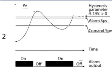
Lower deviation alarm value of alarm setpoint less than "0" and hysteresis value greater than "0" (Par.29 R.L.H.Y. > 0).\*\*
