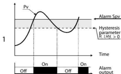
Absolute alarm with controller in heating functioning (Par. 7  $R_{CT.E}$  selected  $HEAT$ ) and hysteresis value greater than "0" (Par.29  $R.I.HY. > 0$ ).\*
