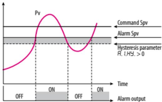
Upper deviation alarm value of alarm setpoint less than "0" and hysteresis value greater than "0" (Par. 64  $R.I.HY. > 0$ ). \*\*
