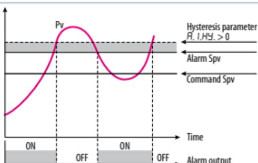
Lower deviation alarm value of alarm setpoint less than "0" and hysteresis value greater than "0" (Par. 64  $R.I.HY. > 0$ ). \*\*
