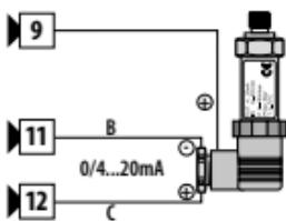
**For signals 0/4..20mA with three-wire sensor**
