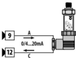
**For signals 0/4..20mA with two-wire sensor**
