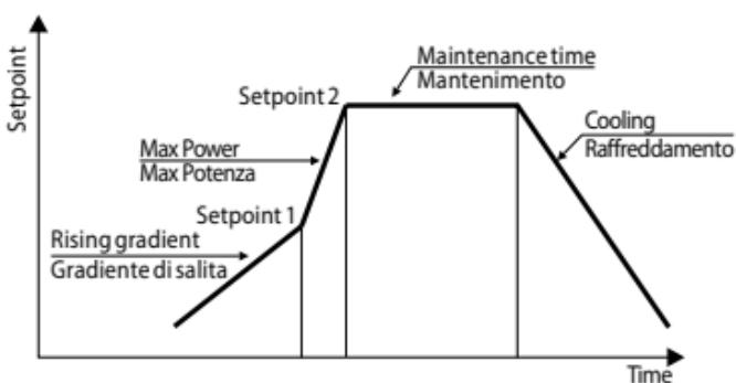
Cycle starts at each activation of the controller, or via digital input if it is enabled for this type of functioning (parameters 94 d.1.F, or 101 d.2.F set as 5E./5E. or RUN).
