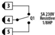
Capacity 5 A / 250 VAC for resistive loads.
