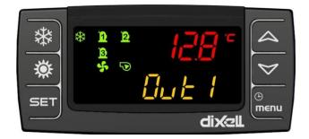
**Fig.2**: upper display shows outlet 2 evaporator temperature, the lower display shows Out2. Pressing SET key is possible to read the same probe of the first circuit.
