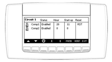
How to reset working hours and number of switching on:
