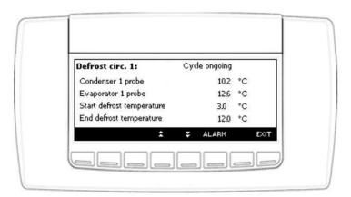
If the combined defrost is enabled, press or to read the probe value and the set point.
