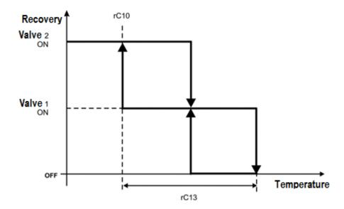
In the heat recovery digital input is active and if the heat recovery temperature is lower than the first valve activation threshold, the recovery valve will be activated on the circuit switched on.
