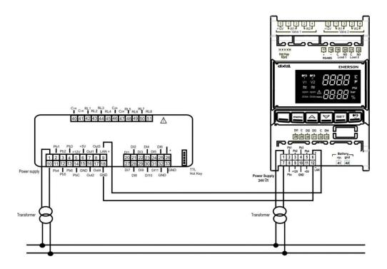
Connection with the same transformer (the power supply of the Ichill and expansion I / O must be 24 Vac/dc).
