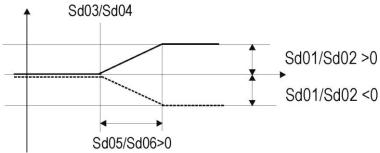
Analog input configured as outside temperature and negative differential:
