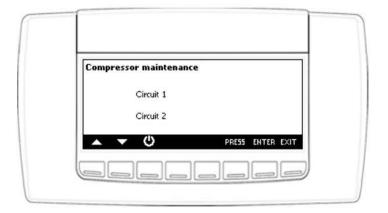
Pressing it is possible to enter on the visualization of the working hour and number of start up of each compressor.
