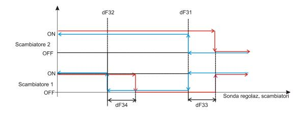
If the machine is switched on and external temperature or condenser temperature/pressure is inside the differential:
