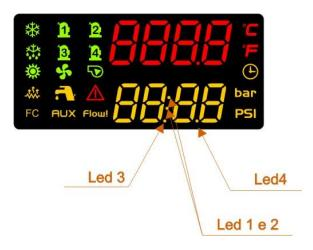
• Leds 1 / 2 are blinking: the parameter can not be changed.
