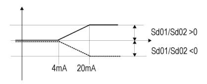
Analog input configured as outside temperature and positive differential:
