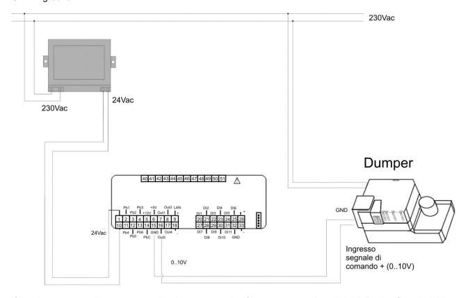
If the dumper motor has a common line between a pole of the power supply and the "-" pole of the 0..10V signal, it is necessary to use two transformers for the power supply of the controller Ichill and the power supply of the dumper motor.
