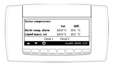
To read the discharge temperature, the status of the liquid injection valve and the status of the minimum load start up valve:
