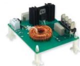
**CW15-KIT e CWC15-KIT:** Ichill wiring kit for 5 realys model and 4 relays + 1 triac model
