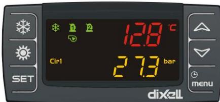
**Upper digits (red color):** configurable by parameter CF36 (PB1, PB2, PB4, Set-point (parameter value)\*, working set-point (real set-point modified from dinamic set-point, Energy saving or function for units without water storage tank), Hysteresis, Machine status \*\*)
