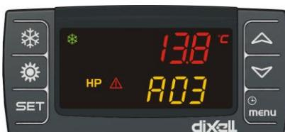
When the instrument detects an alarm, the lower display shows the alarm code alternated to probe value. The alarm icon ( $\Delta$ ) is on flashing.
